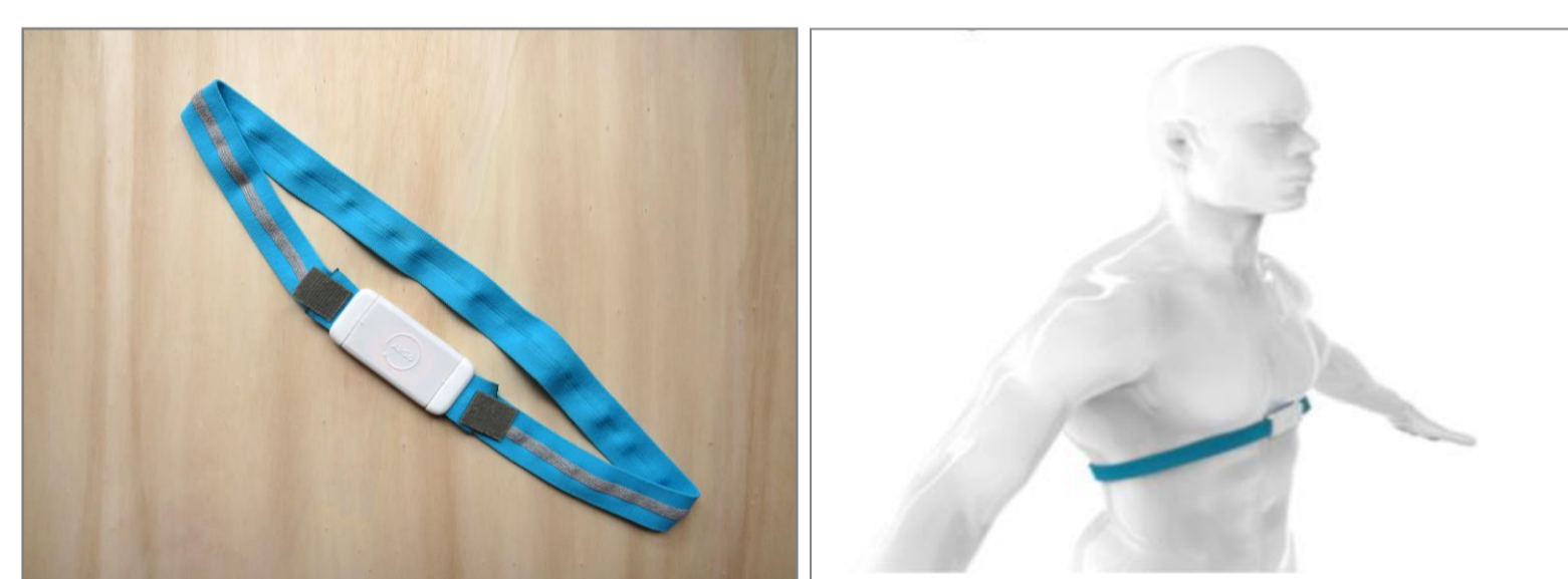
Figure 1: The AirGo™ system (on the left): the stretchable, knitted chest band and the electronic device. The correct positioning of AirGo™ around the subject's torso (on the right).
